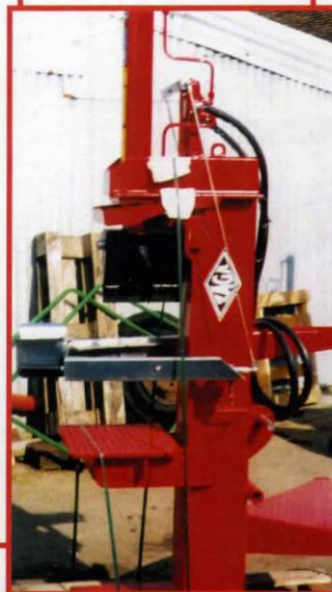
Model OM18HD/CD Showing massive chassis member C/W Integral Hydraulics built in
