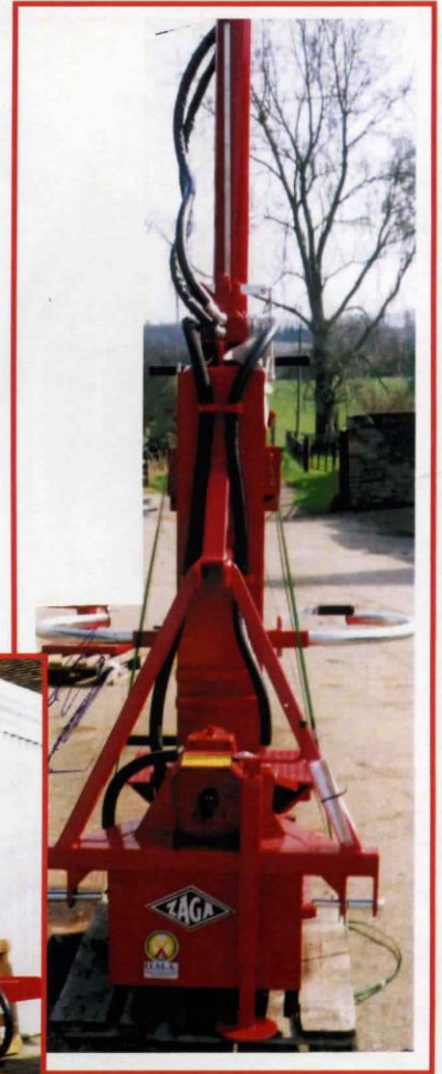
Model OM18HD/CD Showing massive chassis member C/W Integral Hydraulics built in
